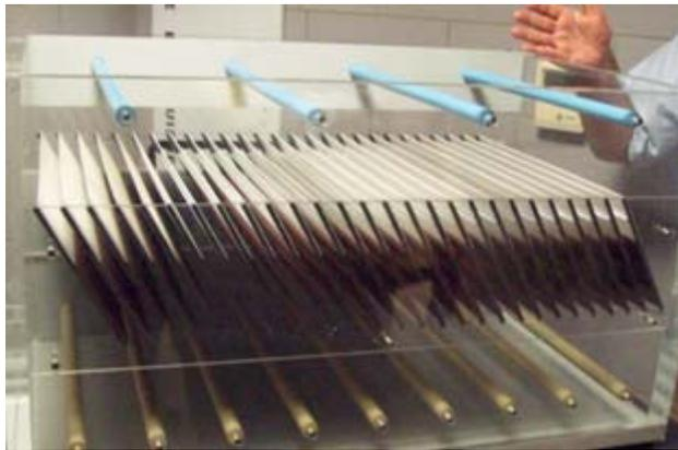
**Scale model of a superpulserator**
